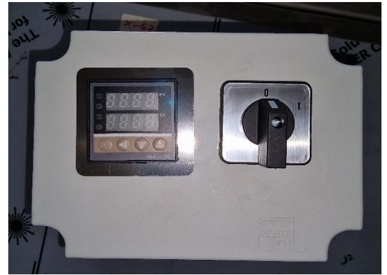
Picture 6. Heating controller
